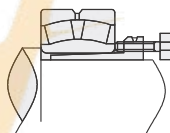
Fig. 9 Removal of Withdrawal Sleeve Using Withdrawal Nut
