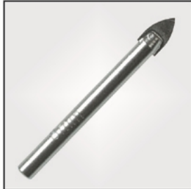
Glass Drill Size: \phi 4.0 \sim \phi 12.0 Material: YG8 Tip
